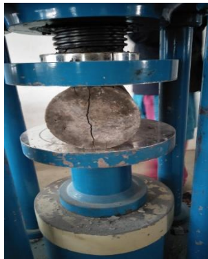
Figure 3 split tensile strength test
