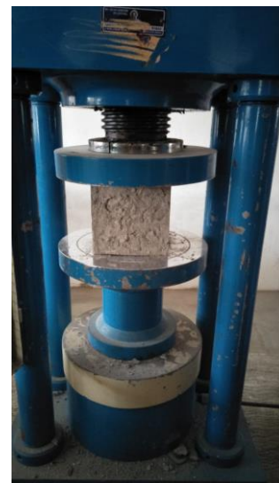
Figure 2 Compressive strength test
