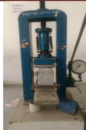
Figure 4 Flexural strength test
